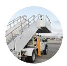
The Airport purchased an Air Stair Truck to facilitate emergency ingress to commercial aircraft containing passengers, but not located at a loading bridge.
